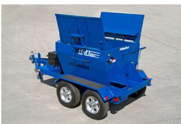
This 2 ton capacity asphalt hauler is ideal for small to medium sized patching jobs. The heated vat is fully insulated for optimum efficiency. The chute-type vat design allows the hot asphalt to be deposited closer to the shoveling platform to reduce operator fatigue.
